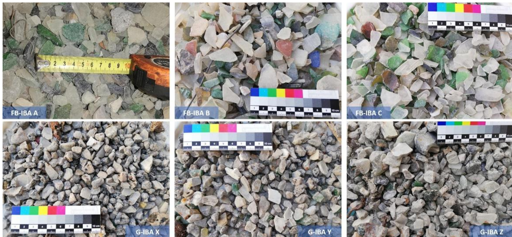
Figure 7: Sensor-based separated glass-fractions 8–35 mm from incineration bottom ashes from fluidized bed (top) and from grate (bottom) – demonstrating optical quality variation between different incineration systems.
